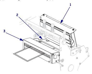
9. Extend approximately 36 in. (920 mm) of media out of the printer. Remove and discard the labels from this exposed media.
